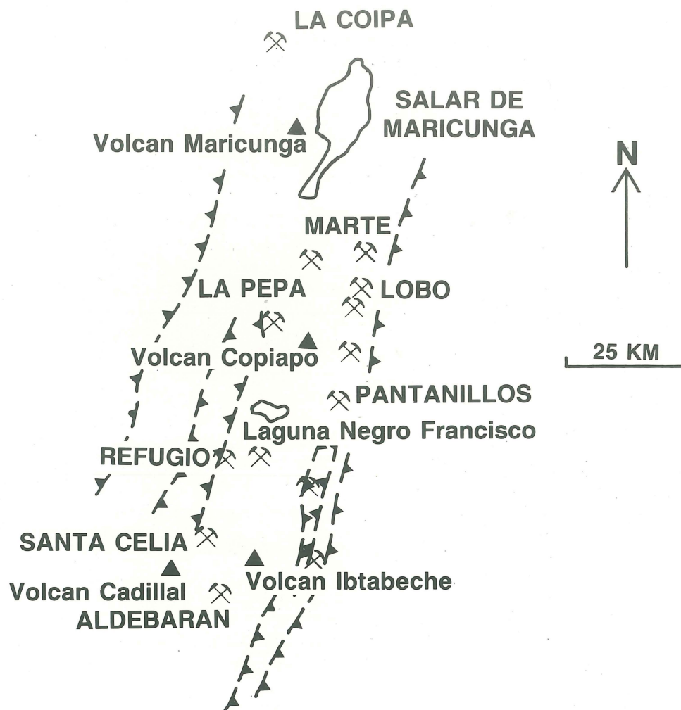
Figure 3. — Location of ore deposits in the Maricunga district, northern Chile. Mine symbols indicate location of deposits; faults are shown with teeth on upthrown side.
